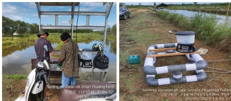
Gambar 47. Setting peralatan automatic fish feeder, digital timer, dan aerator
